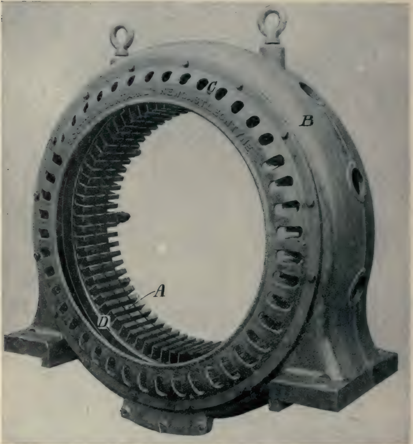
FIG. 4.—Stationary Armature of Alternating Current Motor. Scott & Mountain.
